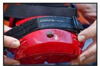
Compare mark on cable with dimples on each side to ensure it is balanced
