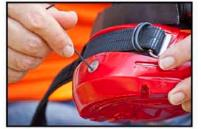
Use allan key to push on clamp to expose screws
