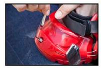
Use allan key to undo screws and release the pressure on the cables
