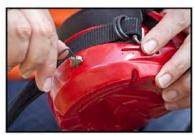
Tighten screws firmly and replace cable clamp into position
